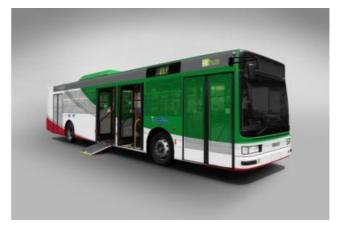
The conversion into hybrid of an old bus with internal combustion engine has two advantages: reducing pollution of our cities and reducing costs and investments. Hybus, in fact, allows to save about 60% if compared with the purchase costs of a new hybrid bus. The revamping also solves the problem of wasting obsolete vehicles, since they can get back on the road with an up-to-date and eco-friendly small displacement diesel engine also boasting an environmentally friendly look.
